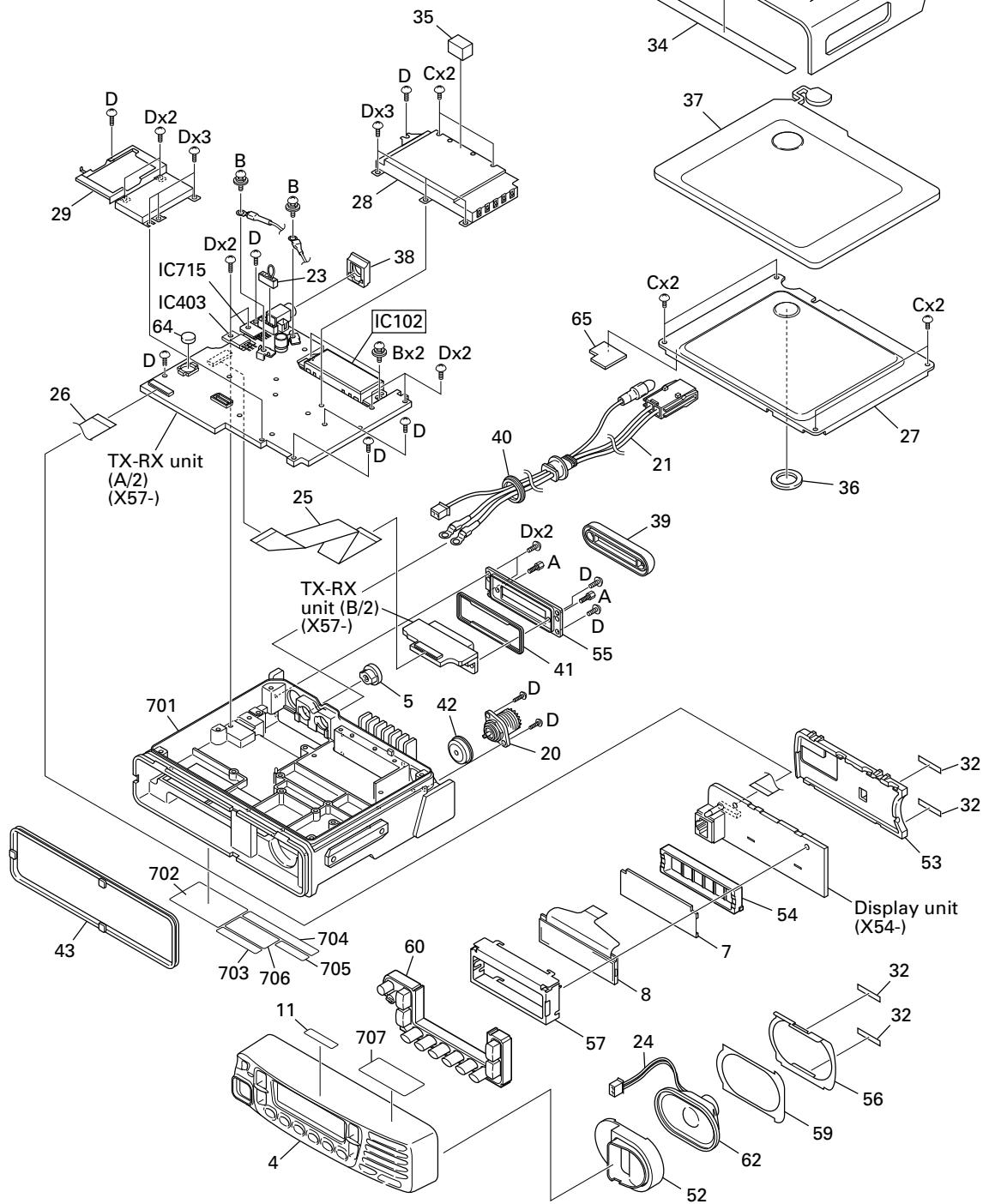
Parts with the exploded numbers larger than 700 are not supplied.
